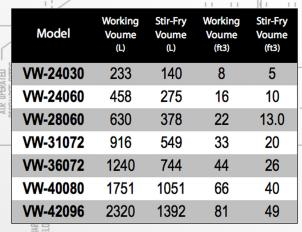
\*Working volume measured to top of agitator. Stir-fry volume is de-rated 40%.
